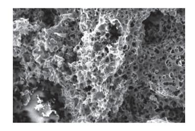
In gas masks, air filters, cosmetics, medicines, water treatment and countless other applications, the enormous absorption properties of the millions of nanopores in each gram of this material has amazed scientists.
