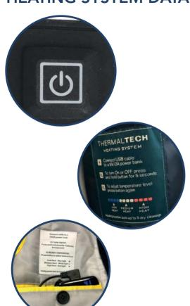
Description: The heating system operated through carbon threads, which are stitched into a carbon fiber felt for the optimal heat distribution throughout the surface area of the heating patches. A silicone encased and illuminated control button, which can contain the logo of our customers, Operates on three different selling. The red color is maximum, white is medium and blue is low.
