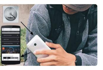
KC Textil has developed a way to integrate NFC chips and antennas into clothing accessories, such as buttons and patches. In this way the NFC technology can become a permanent part of garments, enabling fashion brands to communicate with consumers like never before.
